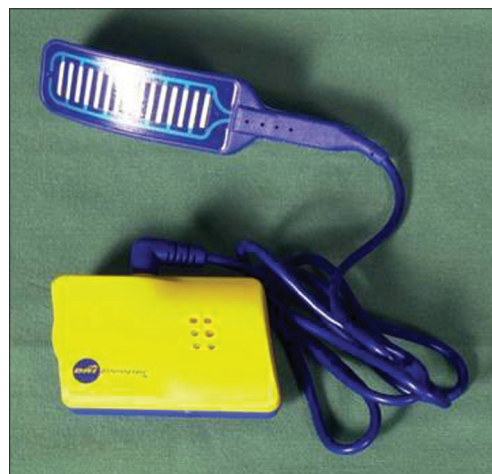
Figure 1: 'Blood leak detector': 'Enuresis pad' between cannulas to detect blood leak. DRI-Sleeper(TM) [flexible], Alpha Consultants, Nelson, New Zealand ( http://www.dri-sleeper.com/ )
